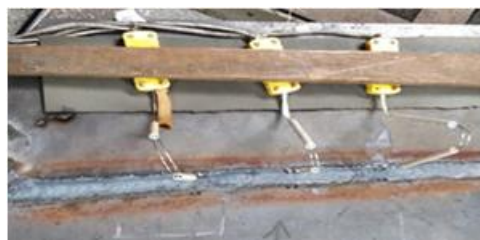
Figure 1: Indicating the Thermocouple weld at different location
